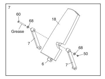
Grease an M14 x 180mm Bolt (60). Attach the Pivot Tubes (7) to the Frame (1) with the Bolt, two M14 Washers (68), and an M14 Nylon Locknut (50). Do not overtighten the Nylon Locknut; the Pivot Tubes must pivot easily.
